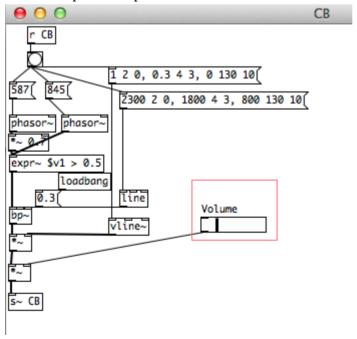
In that patch, you can see that the base signal is a phasor, i.e. a saw tooth signal. The rest of the patch is rather similar to the others.
