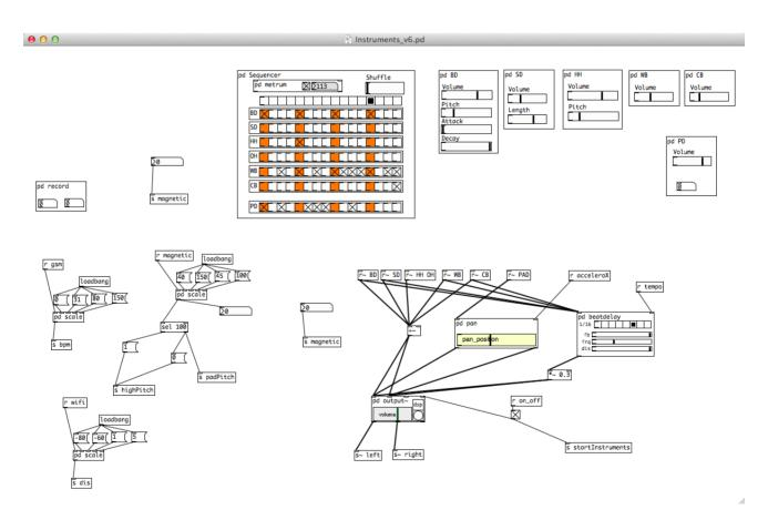
The main part is the beat grid, which controls when the different instruments are played. The different sensors of the phone interact with the parameters of the sound as following:
