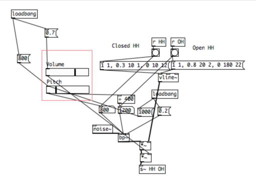
This time, the base signal is not a cosine signal but a white noise, which simulates better the sound of a cymbal. You can modulate the pitch through a band pass filter (bop~). You select if it is a closed hihat or an opened hi-hat by changing the envelope.
