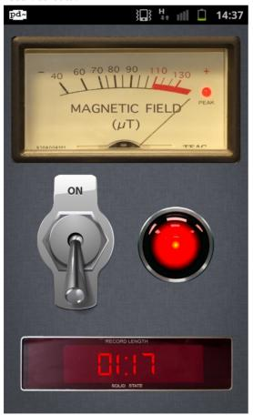
Both buttons are simply two images that exchange places according to the state of the button (pushed or not). The counter is one background image with numbers displayed over it in a font, which imitates the old digital alarm clocks.
